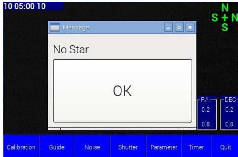
In this case, try increasing the exposure time using [Exposure/Gain] or decrease the star brightness threshold with [Star bright level].
