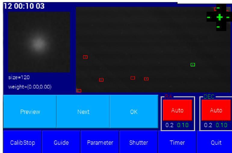
Red boxes indicate potential guide stars. Automatic selection of the best star is highlighted in a green box. Press [OK] to start guiding or just wait for 3 seconds, after which the guiding automatically starts.
