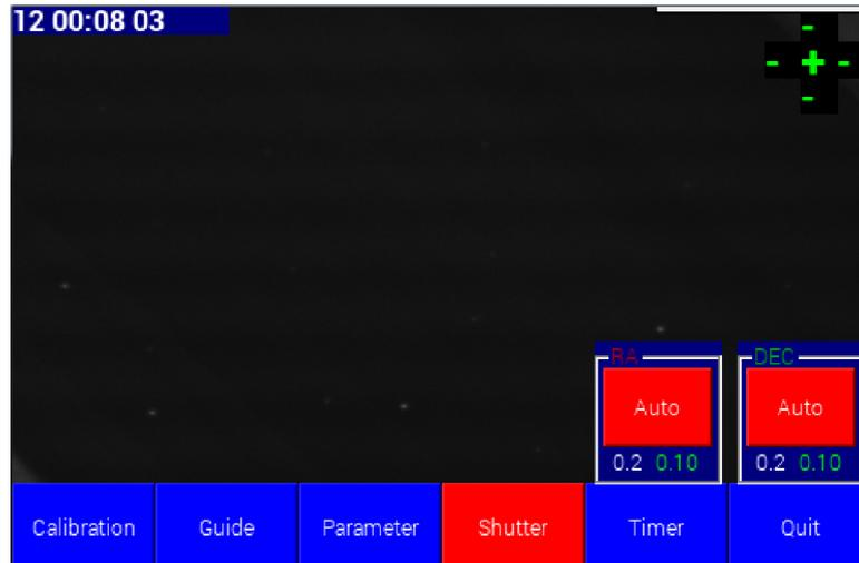
During exposures, [Shutter] alternates between red (shutter open) and yellow (inter-frame delay). Press [Shutter] again to stop imaging.
