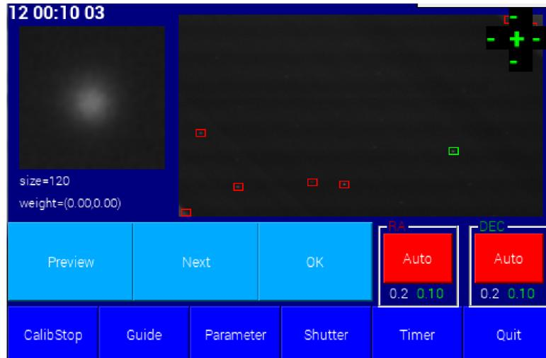
In the upper right quadrant of the display, red boxes indicate potential guide stars. The green box is the best star selected by the controller. Press [OK] to immediately proceed with calibration or just wait for 3 seconds, after which the calibration automatically starts.
