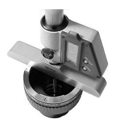
Once the camera measurements have been taken, the focuser must be adjusted to match. The flange-to-knife-edge distance must be adjusted until the measured distance matches the distance derived above. Note that the action of locking the knife-edge in place may cause a slight shift in the final distance, so taking several measurements after locking the position of the knife-edge holder is recommended.
