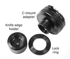
As shown at right, the locking ring and knife-edge focuser screw onto the C-mount section of the Kenko adapter. To adjust the flange-to-knife-edge distance, the knife-edge holder is screwed in or out, and the locking ring is tightened against the holder once the correct position has been set.
