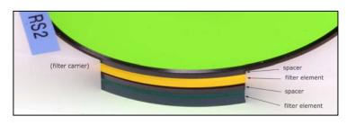
The single-layer filters (L and R) are also supplied with two spacers, one above and one below the filter glass. Note that all spacers are symmetrical and identical so they can be interchanged or flipped over with no problem. They are, however, thin and delicate, so they should be handled with care to avoid bending them out of shape.
