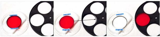
Filter in carrier (left) and filter carousel (right).
