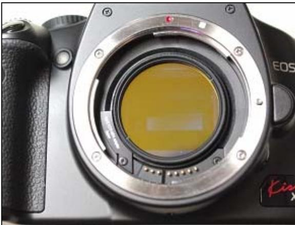
Step 4. Install filter. Screw the IDAS 37mm into the filter holder. **Use only IDAS low profile 37mm filters to avoid damaging the camera body and/or lens.**
