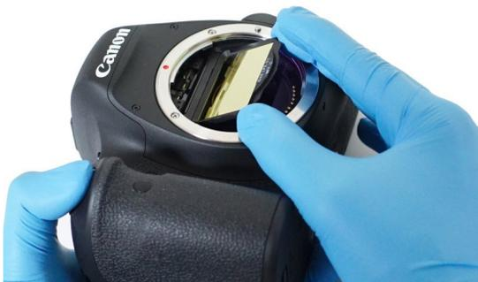
4. Insert a filter while pushing the long edge into the back of the mirror.
