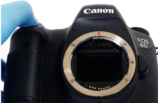
3. Select the mirror lockup item in the menu and press the shutter button to move the mirror up.
