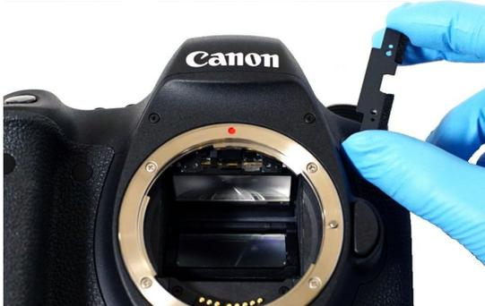
2. Remove the cover. Keep the screws and cover in a storage bag.
