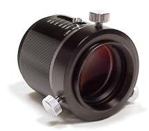
The Borg 1.04X Multi-flattener, part number 7784, is designed for use as a photographic field flattener for 35mm photography with refractors between 450mm and 1200mm. It features a built-in camera rotator ring for easy adjustment of composition, wide non-vignetting light path, and 10 micron spot size out to 90% of the 35mm frame when used with Borg refractors.
