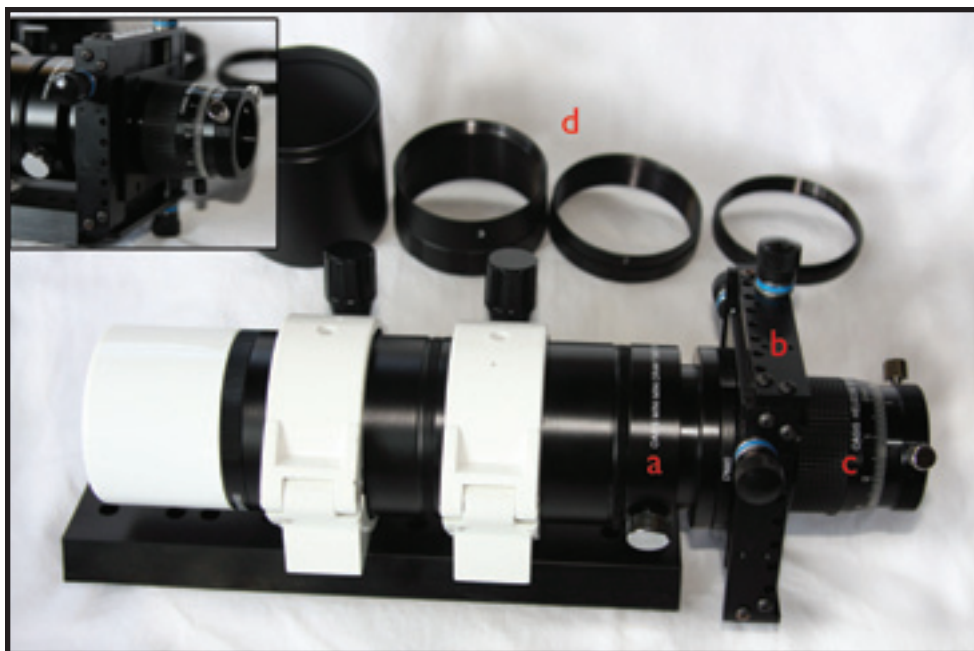
Image 1: Borg guide scope with (a) drawtube, (b) X-Y stage, and (c) helical focuser all attached. For most uses, either the drawtube or the helical fine focuser would be used but not both. Several extension tubes (d) that let you customize the length of the main tube are also shown. Inset shows close-up of X-Y stage and helical focuser. Note, silver set-screws on focuser provide 3-point clamping of 1.25-inch tubes and can be removed to allow a T-mount camera to attach even more securely. The black setscrew on the bottom of the focuser locks the focuser in place.
