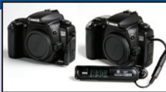
Spectrum-Enhanced Canon 20D with internal thermometer installed. Shown with and without external readout unit attached.
