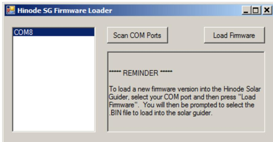
If you have multiple COM ports listed, select the Hinode SG's port before pressing the "Load" button. If you're unsure which port is assigned to the Hinode SG, note which ports are listed in the loader program's selection box, unplug the Hinode SG, then press the "Scan COM Ports" button. The port which has disappeared is the Hinode SG's port. Plug the Hinode SG back in, press the "Scan COM Ports" button again, select the correct port, and proceed with loading the firmware .bin file.
